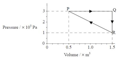
Which of the following is the net work done by the gas in a cycle?
