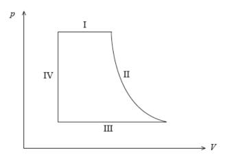
Which of the labelled parts of the cycle identify isobaric changes and adiabatic changes of state?
